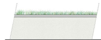
REAR WALL FENCE DETAIL 1/50. 1200MM HIGH BLOCK WALL WITH 1800MM P.C.C. COPING WHERE INDICATED (WALL STEPPED WHERE NECESSARY)
