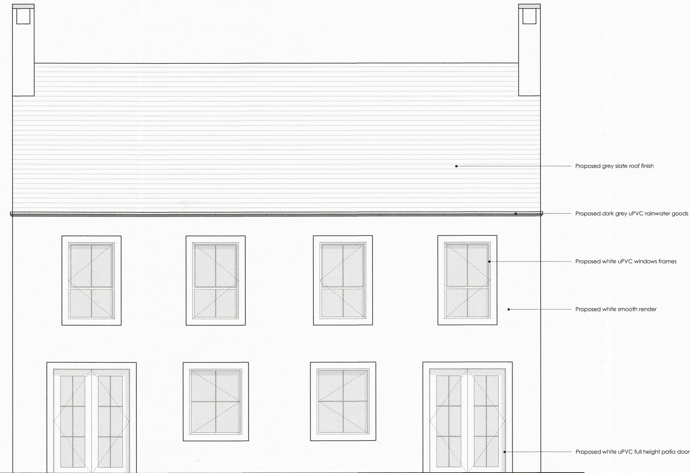
REAR ELEVATION - SEMI DETACHED
