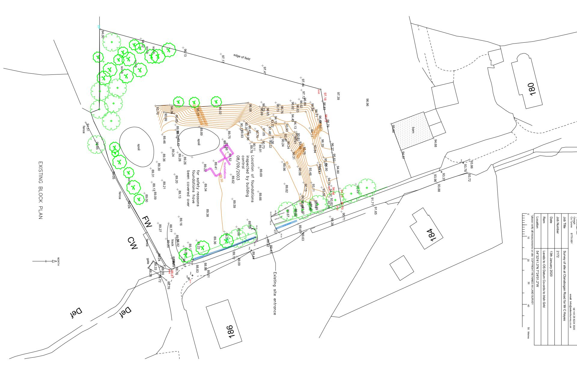
Provide unobstructed sightlines of 45m in both directions direction from the proposed access 2.0m back from the road edge
