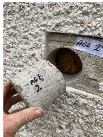
Photograph No2 – Part view of southeast facing elevation showing location of Core Ref AGE 2
