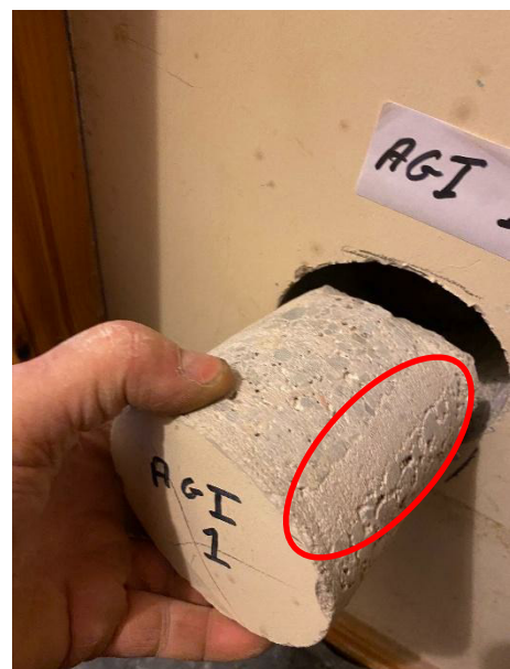
Photograph No 6 – View of internal wall showing location of Core Ref AGI 1. This core was deemed unsuitable for testing due to the presence of a mortar joint
