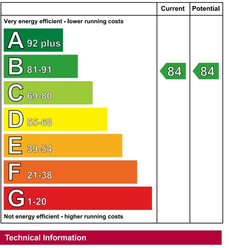
Main heating type and fuel: Total floor area: Primary energy use: Approximate CO<sub>2</sub> emissions: Dwelling type: Boiler and radiators, mains gas 79 m<sup>2</sup> 76 kWh/m<sup>2</sup> per year 14 kg/m<sup>2</sup> per year Ground-floor flat
